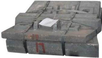
Sag Mill liner from H&G use Cr-Mo materials (AS2074 Standard) , provides superior impact and wear resistance in all semi-autogenous milling applications. The material of SAG mill liners use low or high Carbon Cr-Mo Alloyed steel, the carbon content depends on the working condition of the mill.
